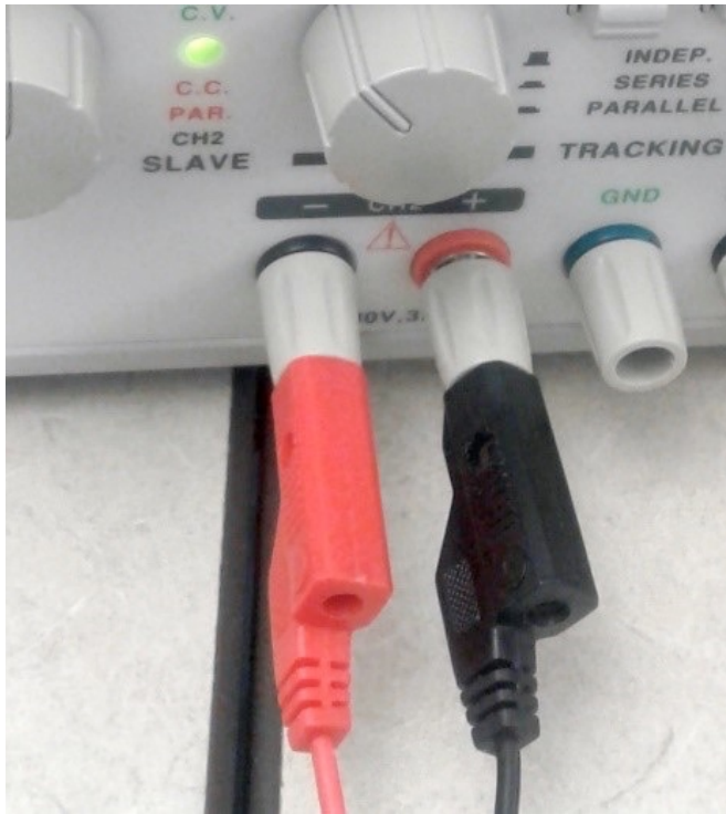
Figure 5: Leads connected in reverse
