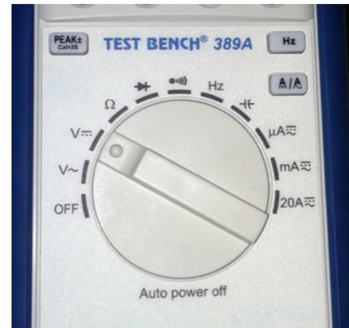
Figure 2: Auto Ranging DMM
