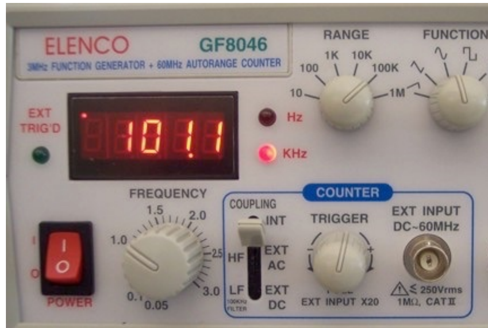
Figure 1: AC Signal Generator with 101.11 k hertz frequency
