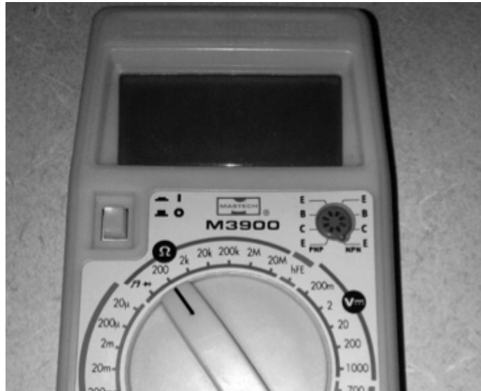
Figure 1: Setting the DMM to measure test lead resistance
