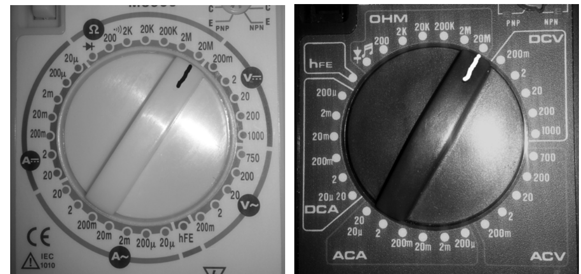
Figure 1: DMM resistance ranges
