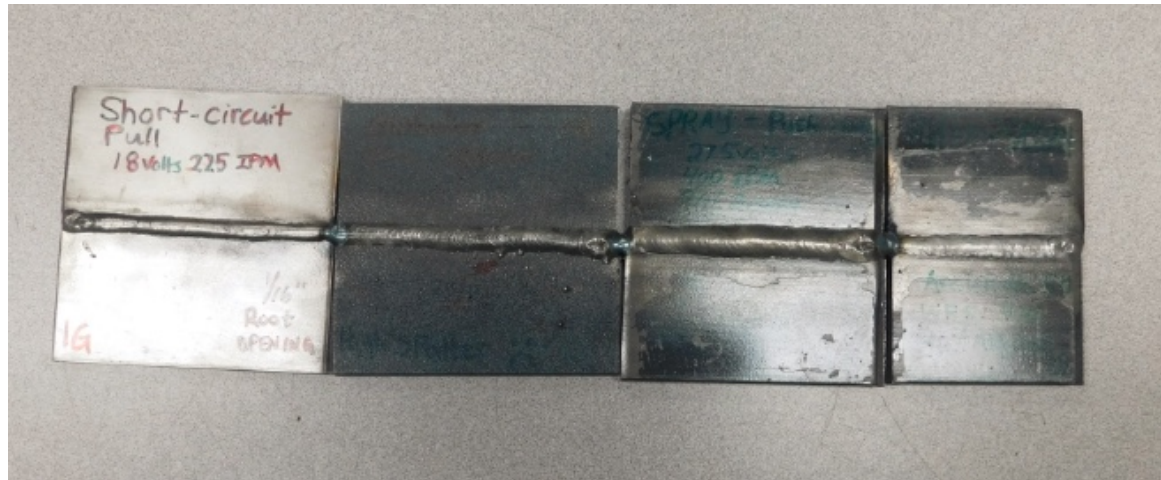
Figure 10: Butt Weld Example
