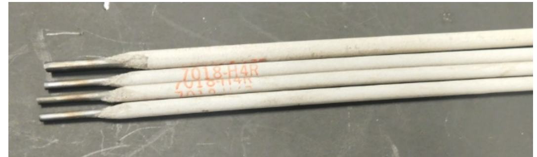
Figure 6: Stick Welding Electrodes - Classification Codes
