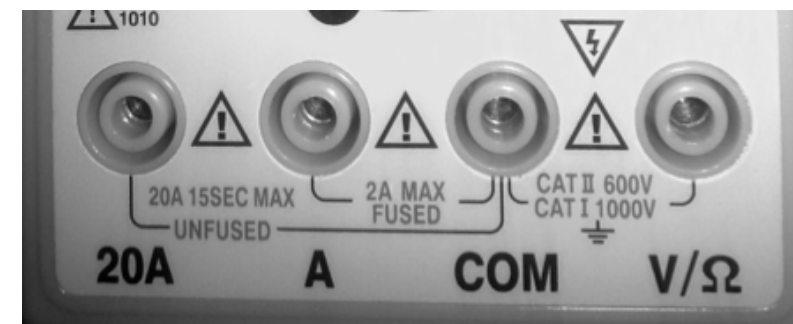
Figure 3: Test lead jacks
