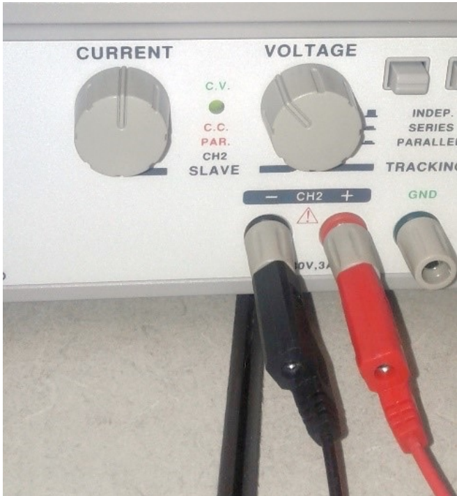
Figure 4: Connecting test leads to the power supply
