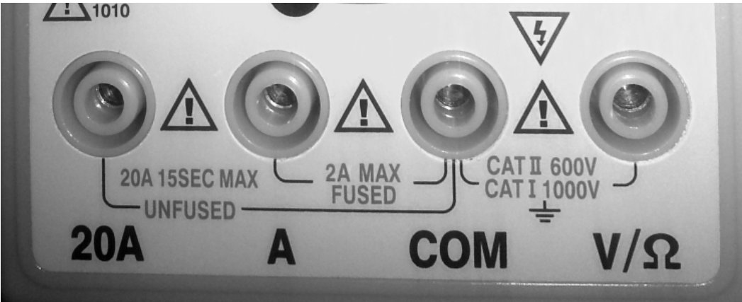
Figure 2: Test lead jacks
