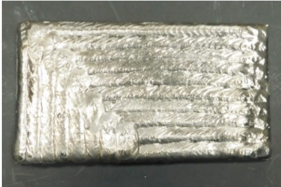
Figure 13: More Overlapping Weld Practice
