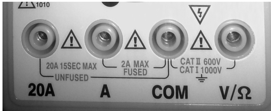
Figure 2: Test lead jacks
