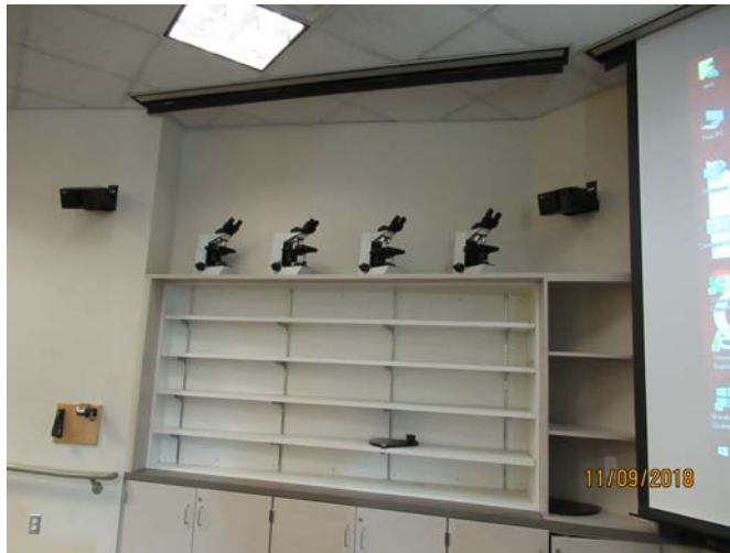
30. Maintain minimum 18-inch clearance between combustibles and ceiling. (with fire sprinklers) CCR Title 8, 6170(b)(10)
