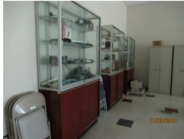
23. Mount display shelves to wall to prevent from falling.
