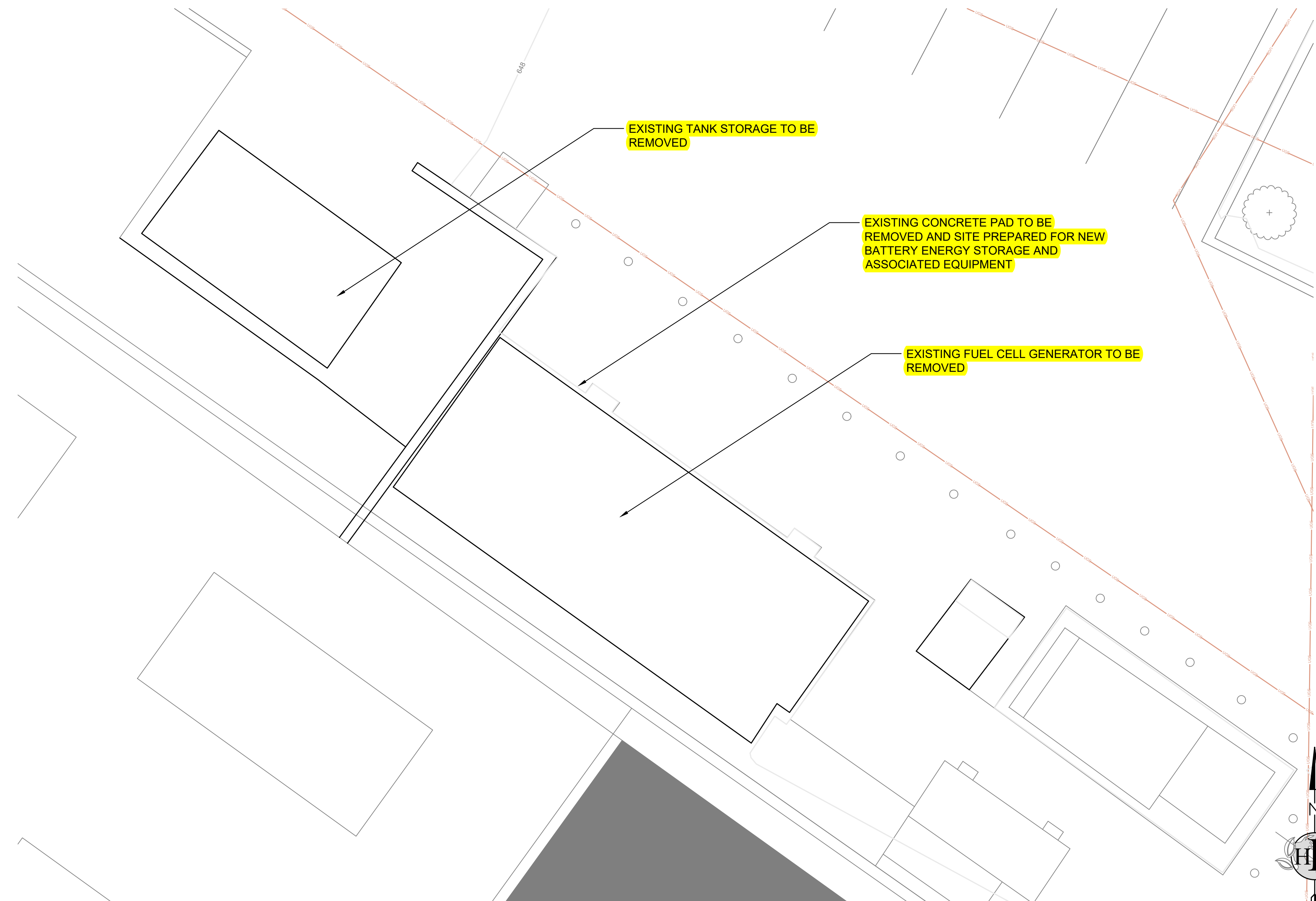
DEMOLITION SITE PLAN - BESS LOCATION
